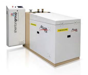
The Micro series benefits from having Tedom's own built in-house high performance gas engines. Available to run on a variety of gas fuels. Multiple units can be run in synch, and high-end digital controllers make synchronising with the mains simple.
