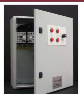
Phoenix dual mains panels are designed to facilitate a dual mains supply to a critical piece of machinery or plant. In the event of supply 'A' failing or going under voltage, the panel will transfer the load to supply 'B', on restoration of supply 'A' the panel will transfer load back to supply 'A'. The Phoenix dual mains automatic changeover panels have been specifically designed to meet building regulations B5 and section 20 of the London building (Act) Amendment Act 1939 and
